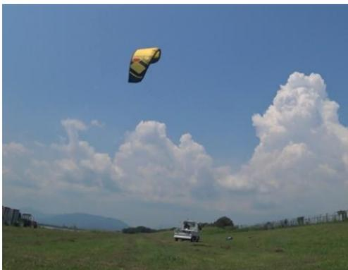
Fig. 3. Truck test of the kite, with the KCU being fixed on the truck body
